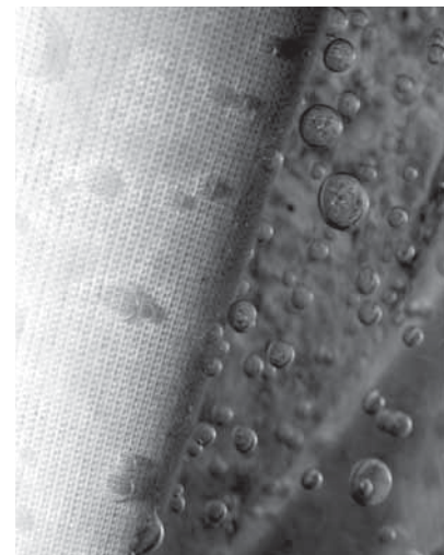
Coalesced water drops releasing from the knitted sock at the outside surface of the cartridge.
